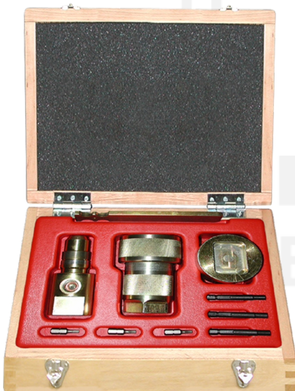
DPE30302 - Injector Tool Kit Tool kit for disassembling and assembly injectors. Also includes an adapter for pop testing nozzles.
