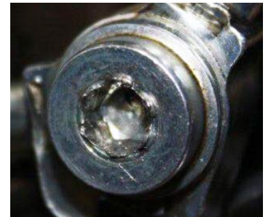
Damaged Banjo Bolt
