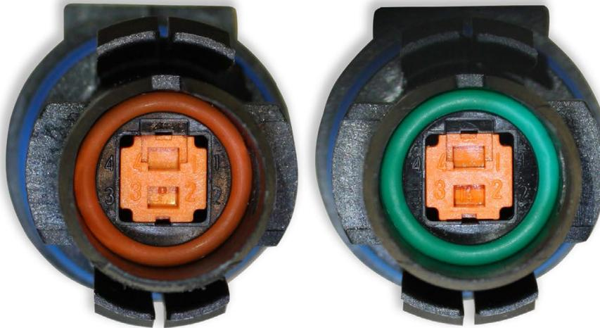
While the color of the seal is different, the reliability of the seal is consistent and will not affect the performance of the injector or the integrity of the electrical connection. The two types of seals may also be intermixed on an engine with no influence on performance.
