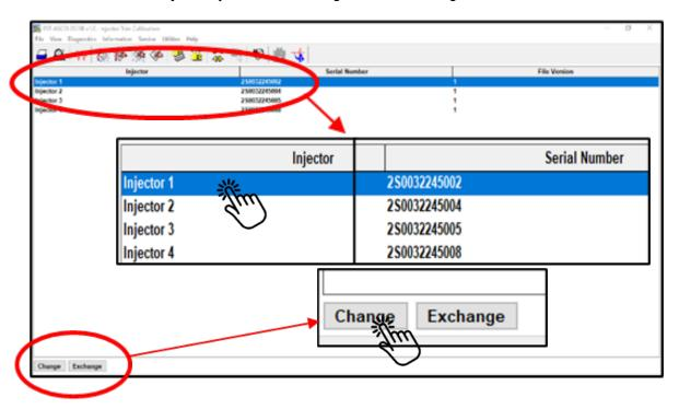
5. After you select *Change* the program will open a Windows box which should display the file from your USB drive which should match the serial number on your new injector. Select this file and click *Open*.
