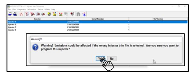
7. Injector programming should now be complete. Repeat steps 1-6 if you have multiple injectors to replace in the engine.
