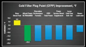
Lowering CFPP temperature of base fuel reduces the risk of fuel gelling and provides superior cold starting and cold weather engine performance.
